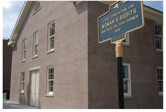
The National Park Service selected the sand weathered texture of Decro Face manufactured in the original size of the 1800's brick. Header brick and special tapered shapes were fabricated for jack arches over the windows:
