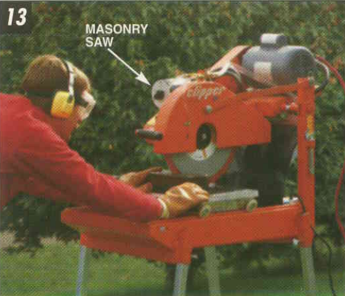
13 CUT PAVERS on masonry saw. Saw has a built-in sliding carriage for moving pavers past the blade. Recirculating water keeps blade cool and lubricated.
