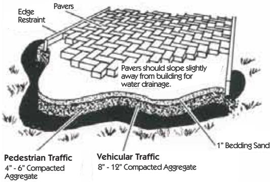
With a properly prepared sub-grade and base, a sand set installation is suitable for all types of pedestrian and vehicle traffic installations.
